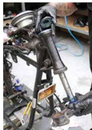
2 Kalby refits the lower triple clamp with new bearings.
