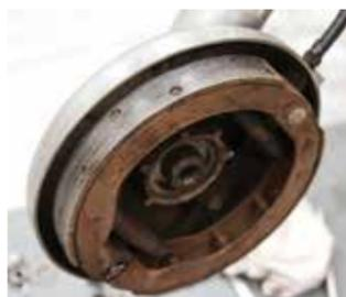
3 The cable operated front brake had a reasonable amount of brake shoe lining left so it was cleaned up but otherwise left alone.
