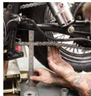
10 After fitting the new chain Kalby shows me the required amount of slack to ensure proper function.
