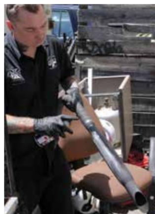
6 After wrapping the highly modified pipes Kalby sprays the muffer sections with heat resistant black.
