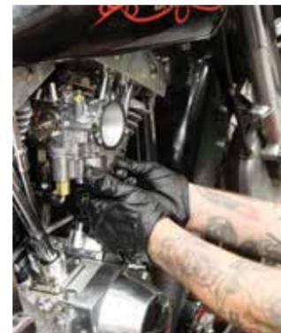
11 Before the first start up Kalby checks the jetting of the S&S carb.
