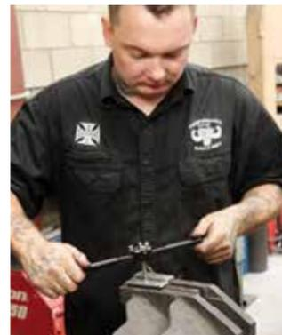
8 Kalby threads some steel stock to make mounting bolts for the exhaust.
