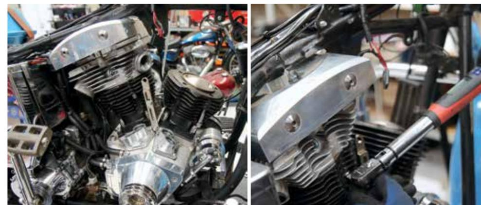
ABOVE LEFT: After putting a new gasket in place Adam places the rear head into position. ABOVE RIGHT: And now begins the process of tightening it to specifications. BELOW: Now he begins the task of fitting new spark plugs and hooking up the spark plug wiring. INSET: New Ultima ignition module.
