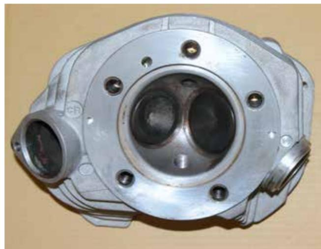
solutions. Andy suggested that we begin addressing this difficulty by fitting manual decompression releases in the heads, which should make it much easier to kick over. For those of you unaware of how these units function, what they do is vent high cylinder pressure to reduce the associated high starter torque required to turn the crankshaft when starting the engine.
