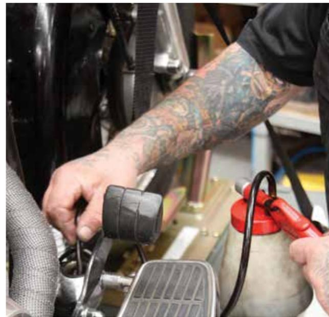
ABOVE: Andy removes the old brake fluid from the master cylinder.
