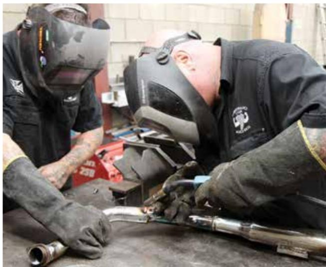
ABOVE: The next challenge for the boys was to make major modifications to the header pipes as the Baker 6-into-4 with Kicker is wider than the original gearbox. An entire day was spent cutting, shutting and welding to make this happen.
