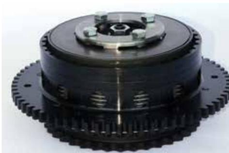
LEFT & ABOVE: Shovel owners know the sad story. The torque on the clutch nut backs off a hair and the key on the transmission mainshaft shears off. This usually happens at the most inconvenient time and place. The Baker splined Shovel clutch kit retrofits and upgrades the stock tapered mainshaft and clutch to a modern 18-tooth spline configuration.
