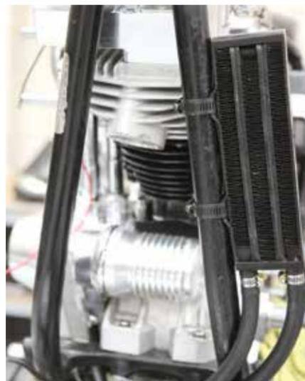
LEFT: Because the bike will be ridden in the Northern Territory as well as across the Nullarbor we decided to fit an oil cooler, which also came out of my old parts stash. Following the mounting of the cooler Kalby cut and fitted oil lines to suit.
