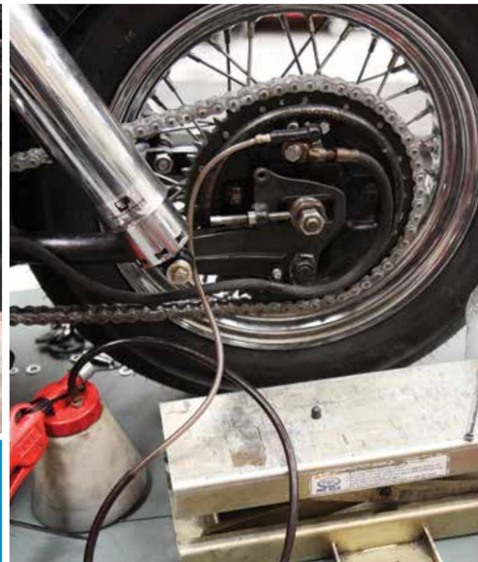
RIGHT: The rear wheel brake cylinder needed to be replaced and after re-assembly, the system is then bled. Now we're getting close and there aren't that many steps to go in getting the old girl ready for the long road ahead. I can tell you, my excitement is really building now.
